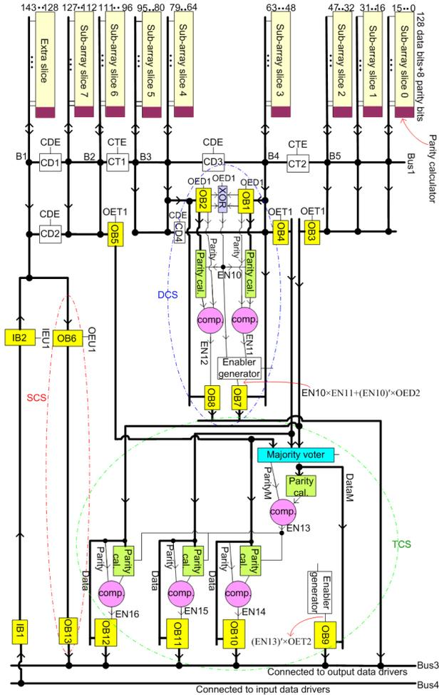
Figure 1: Sub-array block diagram.
